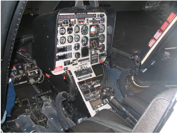
Cockpit of NJSP N6NJ (Bell) showing the 800 MHz radios on the co-pilots (left) side. The VHF radios are on the center console.
